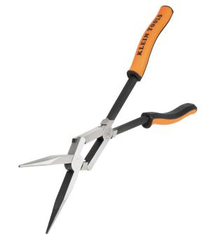
The Klein Tools 13-Inch Long Reach Pliers are designed to improve access into tight spots across a variety of applications. The dual rivet design allows the jaws to open faster than the handles, ensuring the ability to grip on a workpiece without obstruction. These feature straight jaws with Klein's unique angled knurls to provide an extra grip that limits slippage.
